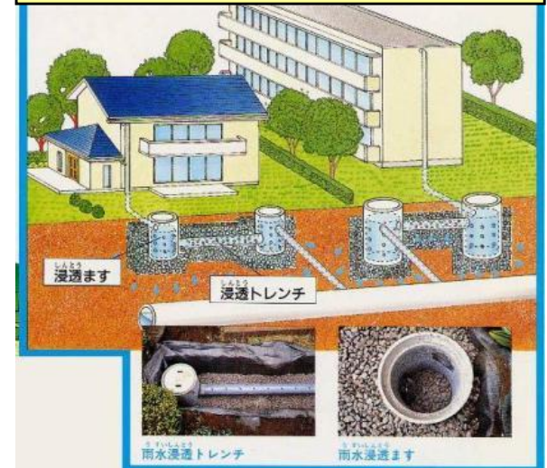
Infiltration trench and inlet
