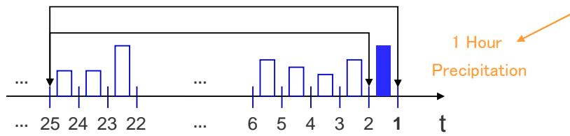
$$Q_{\text{sur}}(t) = \frac{\left( \sum_{t=1}^{24} P(t) - 0.2S \right)^2}{\sum_{t=1}^{24} P(t) + 0.8S} - \frac{\left( \sum_{t=1}^{23} P(t) - 0.2S \right)^2}{\sum_{t=1}^{23} P(t) + 0.8S}$$
