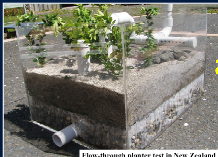
Flow-through planter test in New Zealand
