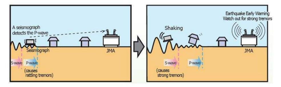
The EEW system automatically calculates an earthquake's focus and magnitude from P-waves detected near the epicenter, and then estimates the intensity of expected ground shaking (seismic intensity) at numerous locations in cities, towns and villages. An EEW message is provided a few seconds to a few tens of seconds <u>before S-waves, or</u> <u>strong tremors, start</u>.
